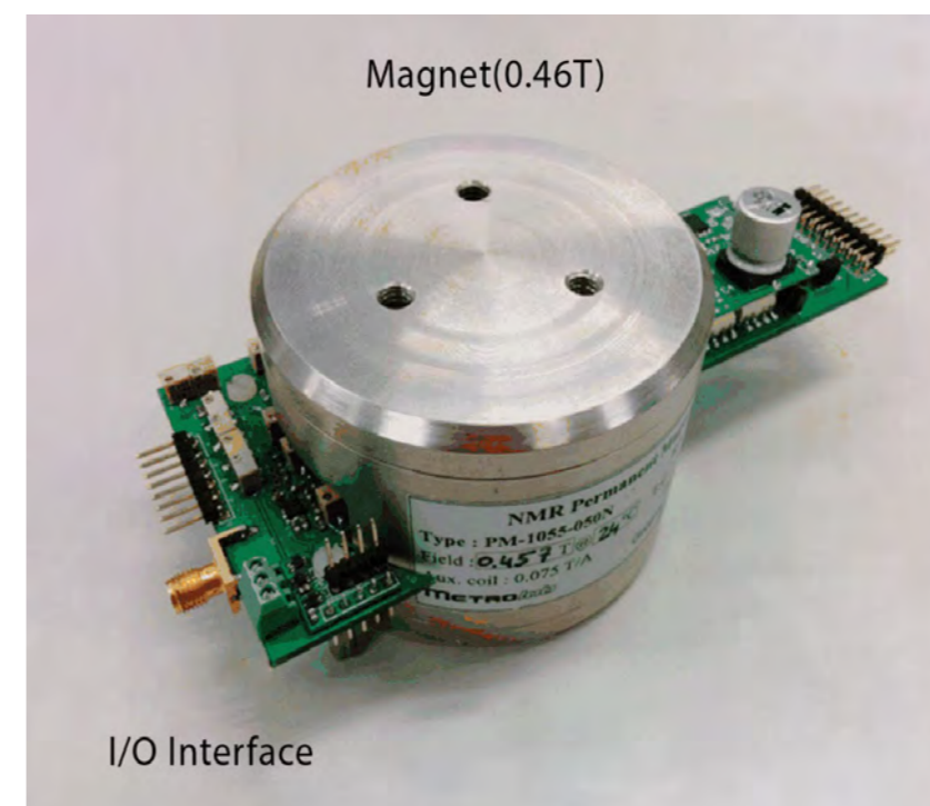
圖三： 第一代可攜式核磁共振系統，其CMOS芯片安裝在磁鐵內的印刷電路板上。 1 Picture 3: The system hardware of our first portable NMR system. The CMOS IC is mounted on the printed circuit boards and put inside the magnet 1 .
