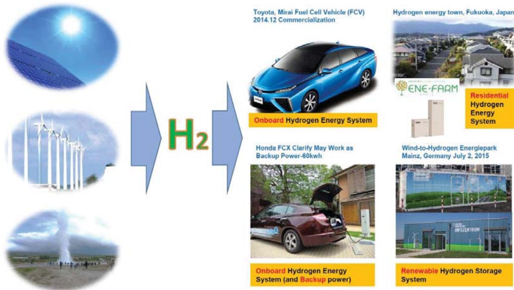
Figure 1. A scenario of hydrogen energy society. Hydrogen can be produced from various energy sources, especially from renewable power. Through fuel cell energy conversion technologies, hydrogen can be utilized for onboard storage, residential applications, backup power, as well as large scale stationery energy storage.
