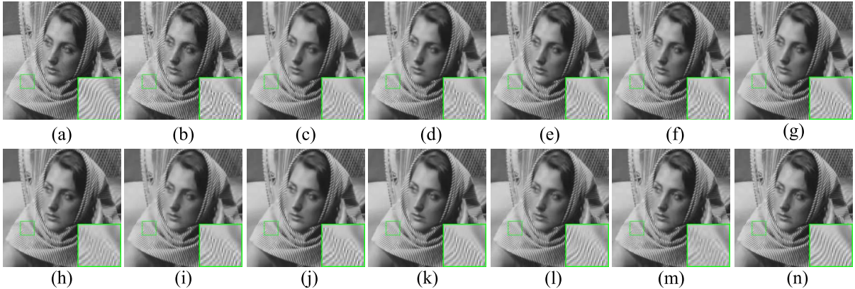
Fig. 8. Visual comparison results of image Barbara at QF = 20 . (a) Original image; (b) JPEG compressed image (PSNR = 29.36dB, SSIM = 0.8831); (c) KSVD [2] (PSNR = 30.60dB, SSIM = 0.9021); (d) FoE [35] (PSNR = 30.10dB, SSIM = 0.8964); (e) BM3D [23] (PSNR = 30.70dB, SSIM = 0.9130); (f) SA-DCT [34] (PSNR = 30.36dB, SSIM = 0.9089); (g) PC-LRM [59] (PSNR = 31.13dB, SSIM = 0.9158); (h) ANCE [60] (PSNR = 31.27dB, SSIM = 0.9119); (i) DicTV [53] (PSNR = 30.67dB, SSIM = 0.8981); (j) WNNM [61] (PSNR = 31.09dB, SSIM = 0.9152); (k) SSR-QC [33] (PSNR = 31.86dB, SSIM = 0.9229); (l) TGV-SH [62] (PSNR = 29.96dB, SSIM = 0.8976); (m) COGL [63] (PSNR = 30.76dB, SSIM = 0.9036); (n) JPG-SR (PSNR = 32.58dB , SSIM = 0.9331 ).
