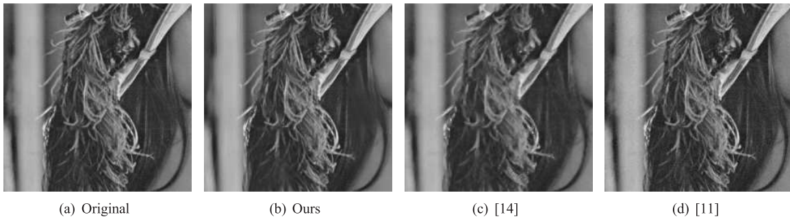
Fig. 14. Visual comparison of image Lena. (a) Original; (b) Proposed (PSNR 33.63 dB, rate 1.5030 bpp); (c) [14] (PSNR 31.46 dB, rate 1.5 bpp); (d) [11] (PSNR 34.6 dB, rate 1.7654 bpp).
