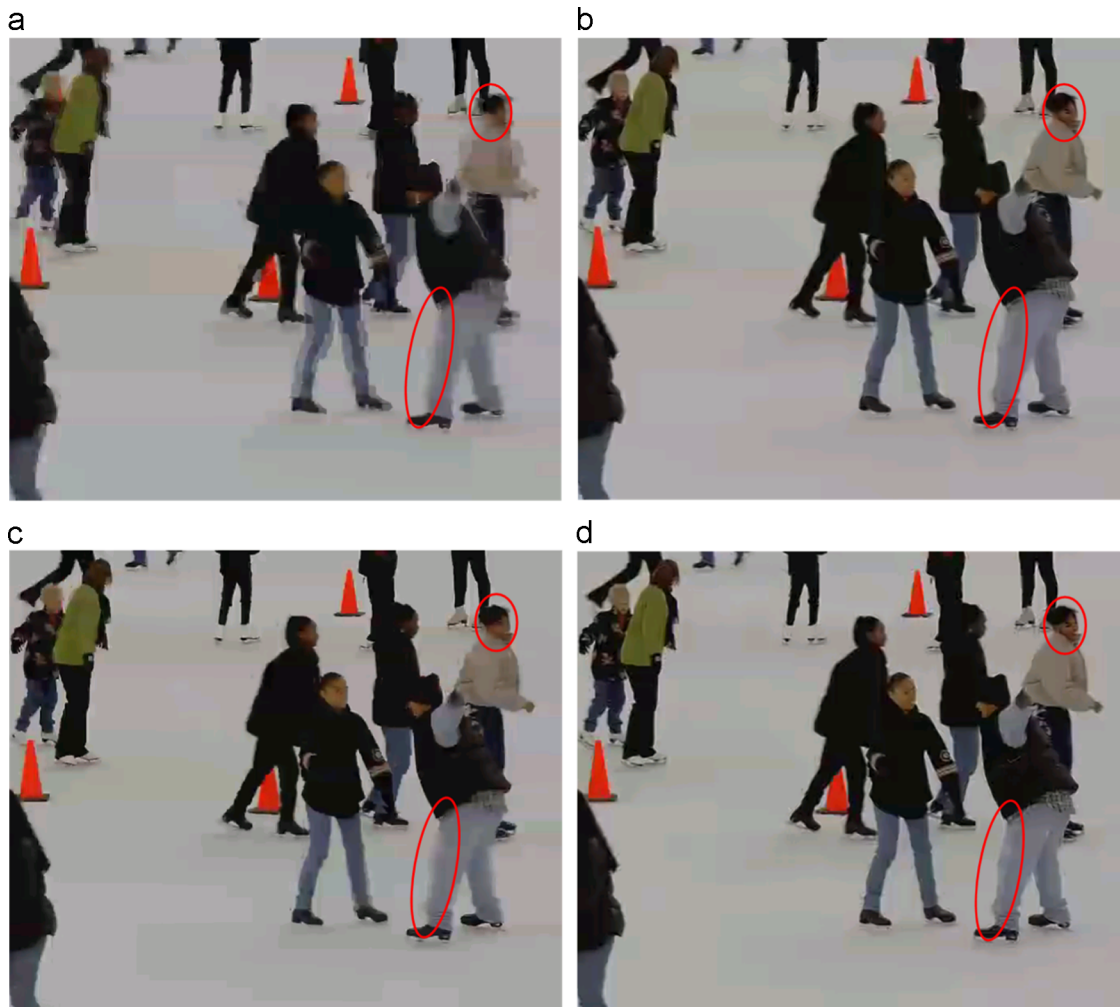
Fig. 7. Subjective quality comparison of the reconstructed second frame in Ice sequence with (PSNR, SSIM, Bit Rate). (a) H.264 Zero Motion (28.68db, 0.8703, 397.27kbps) (b) DBC, (33.01db, 0.9203, 423.76 kbps) (c) H.264-Motion (33.77db, 0.9073, 401.01 kbps) and (d) Our method (33.36db, 0.9259, 413.44 kbps).
