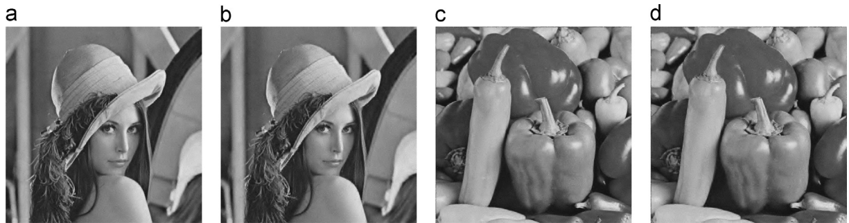
Fig. 8. The reconstructed images and their PSNR values under SR=0.5 : (a) PSNR=32.6432, PLR=0.2, BWHT32; (b) PSNR=31.2287, PLR=0.3, BWHT32; (c) PSNR=32.0629, PLR=0.2, BDCT32; (d) PSNR=30.7208, PLR=0.3, BDCT32.
