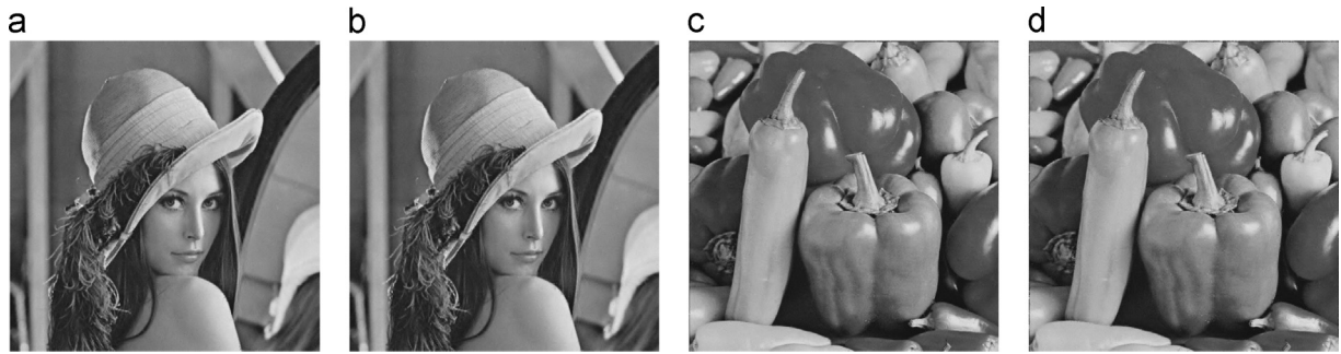
Fig. 7. The reconstructed images and their PSNR values under SR=0.8 : (a) PSNR=35.7965, PLR=0.2, BWHT32; (b) PSNR=33.8944, PLR=0.3, BWHT32; (c) PSNR=35.2942, PLR=0.2, BDCT32; (d) PSNR=33.2762, PLR=0.3, BDCT32.
